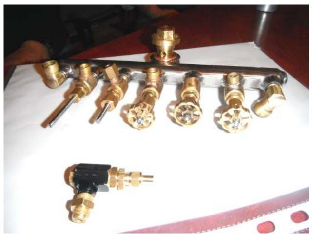
Mark Taylor had a impressive steam turret for his Phantom as well as some check valves plus a set of new piston rings for the A3 Flying Scotsman which he hopes will fix the problems. He showed the fixtures he had made for producing the new rings.
