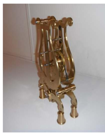
Murray Brown has been making progress with his clock project which is looking very impressive. He has found that piano wire and stainless TIG wire make satisfactory pivots and gears.
