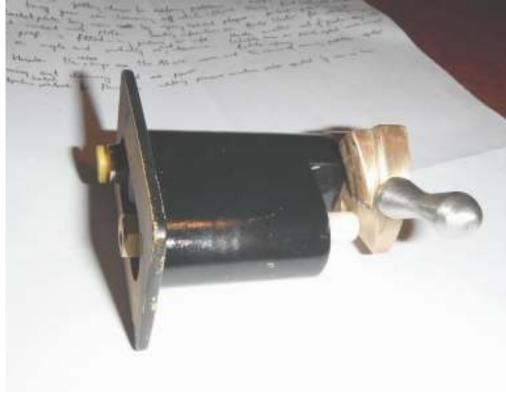
He showed the brake control valve for his Phantom utilising a pressure sensitive valve operated by a cam on the control lever. He showed a video of his visit to the Sydney Society of Model Engineers and their extensive facilities at Ludenham. The complex has trains, boat pond, tethered car track and a flying site.
